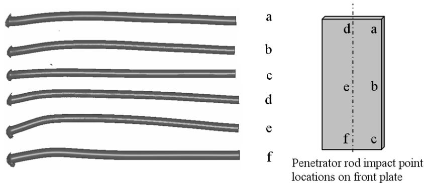
Figure 3. Projectile shapes after interaction with a reactive armor module at different locations on the front plate
