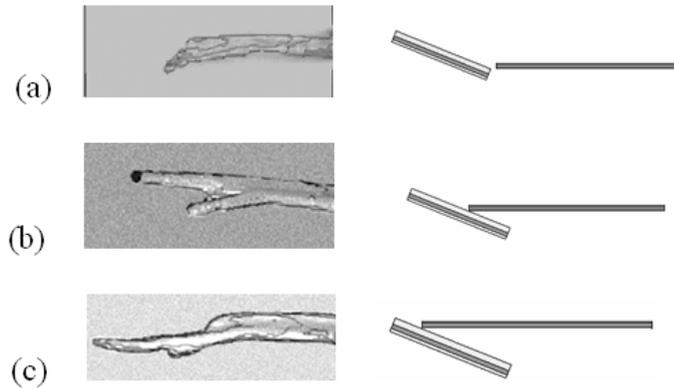
Figure 8. Crater channel shapes for different impact points after penetration into witness plate
