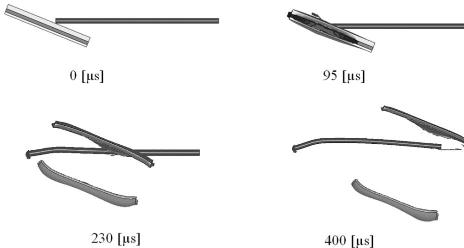
Figure 1. Projectile penetration processes into armor module cassette
