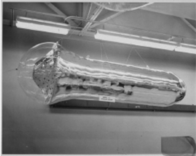
Figure 6-1. Photograph of a US replica decoy for the MARK IV reentry vehicle that was used on some Titan ICBMs. US Air Force photo 113217 USAF, dated 19 October 1961, reprinted from Chuck Hansen, "Swords of Armageddon," CD-ROM (Sunnyvale, Calif.: Chukelea Publications, undated) Vol. 7, p. 560.
