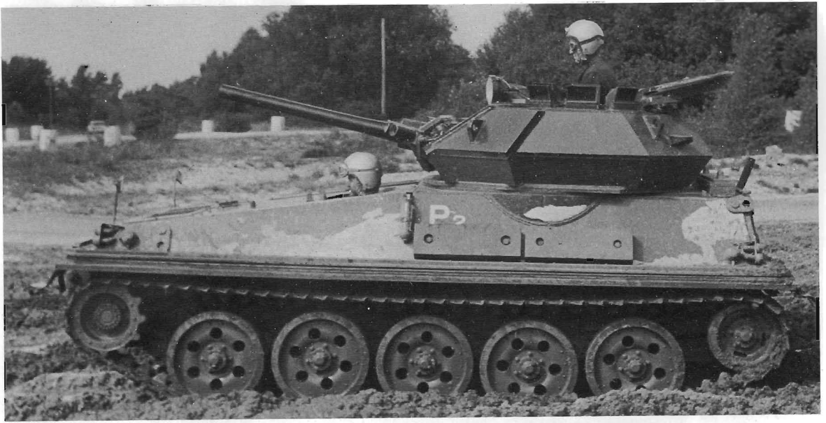
Side view of a Scorpion prototype which illustrates the rear location of the turret (Alvis)
