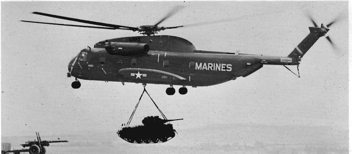
Scorpion lifted by a Sikorsky S-65 helicopter of the U.S. Marine Corps
