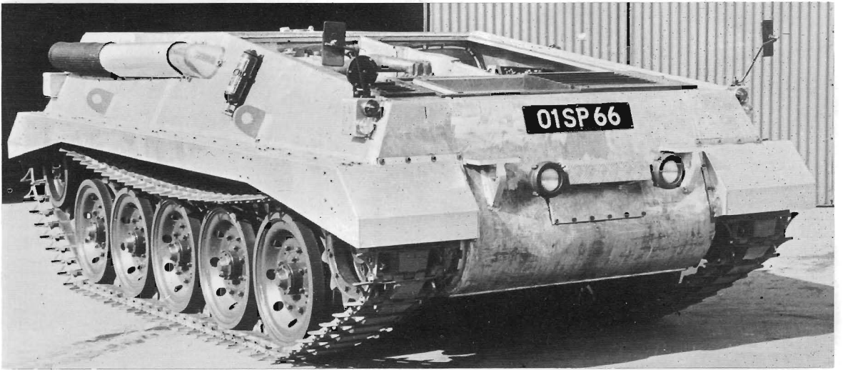
MTR, or Mobile Test Rig, in which the engine, transmission and other components of the Scorpion were tested prior to the construction of its prototypes (MVEE)
