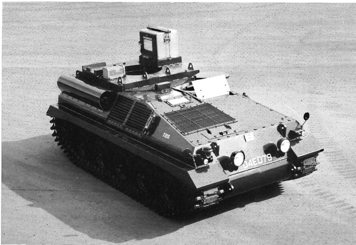
TV 15000, a turrettless test vehicle with instruments to record its performance
