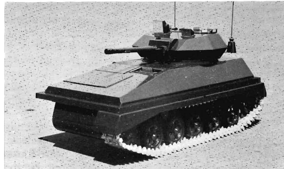
Small-scale model of a very light weight reconnaissance tank proposed in 1964 which clearly foreshadowed the Scorpion; one track has been left off this model. (MVEE)
