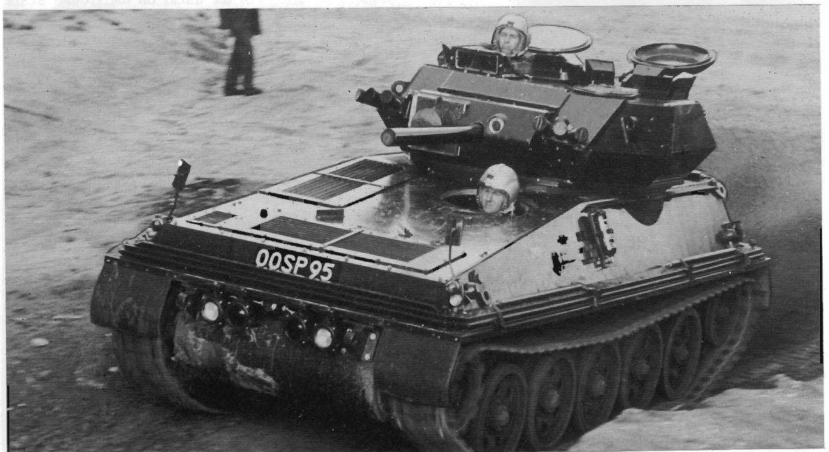
Scorpion prototype, showing the louvres over the engine compartment (Alvis)
