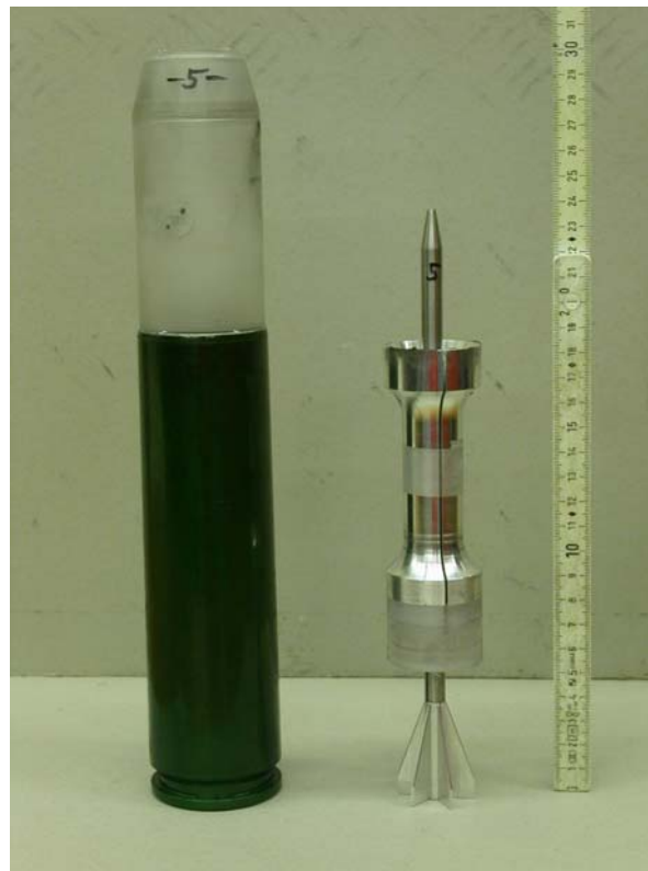
FIGURE 5: L/D 29 MONOBLOC TUNGSTEN KE-PENETRATOR WITH ORIGINAL 35 MM STEELCASE, STRECHTED BY 80 MM APPLYING AN ADD-ON PLASTIC CONTAINER
